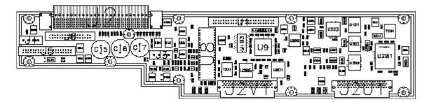
Figure 8-1: Placement Diagram Primary Side
